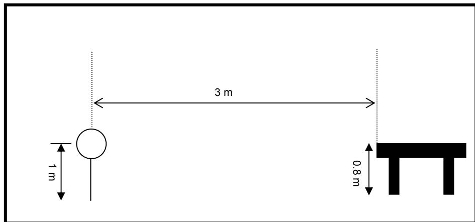
Radiated emission setup, below 1 000 MHz
