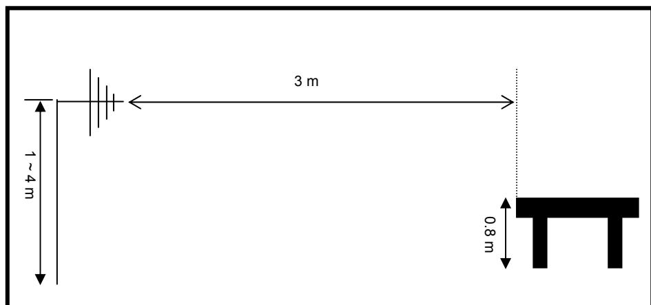
Radiated emission setup, above 1 GHz
