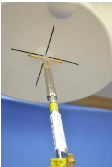
**Construction:** Symmetrical dipole with 1/4 balun. Enables measurement of feedpoint impedance with NWA. Matched for use near flat phantoms filled with brain simulating solutions. Includes distance holder and tripod adaptor.
