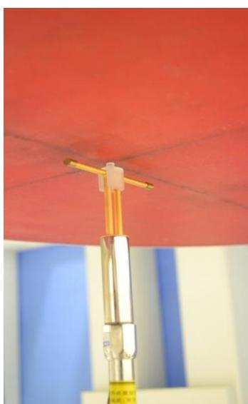
**Construction:** Symmetrical dipole with 1/4 balun. Enables measurement of feedpoint impedance with NWA. Matched for use near flat phantoms filled with brain simulating solutions. Includes distance holder and tripod adaptor.
