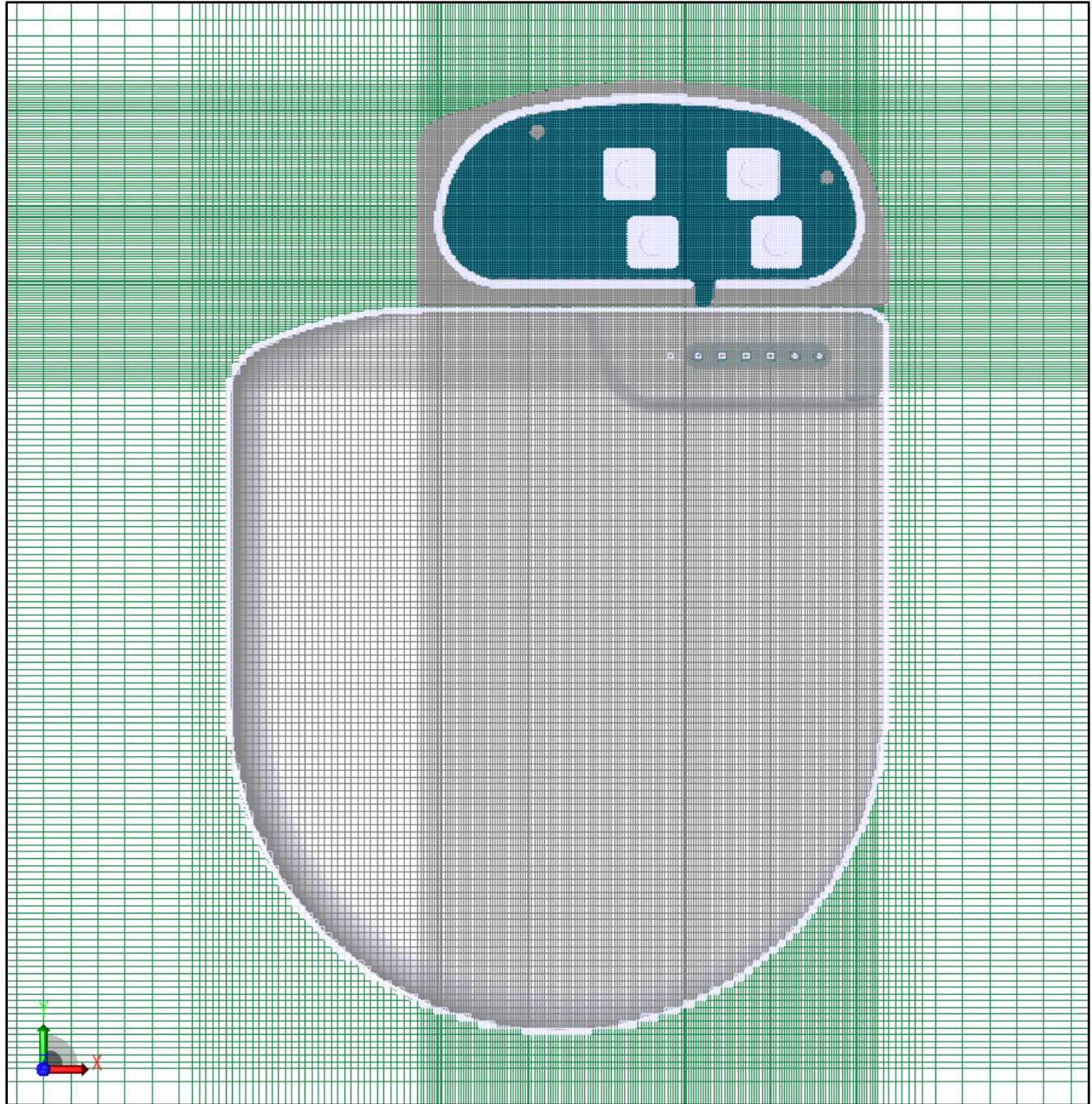
Figure 3 FDTD grid lines showing front of device
