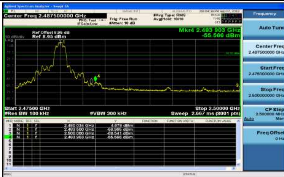
Band-edge for RF Conducted Emissions_3DH5_2402_Hopping On
