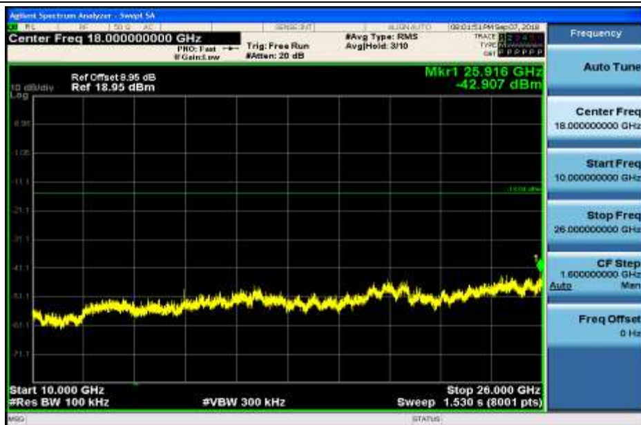
RF Conducted Spurious Emissions_2DH5_2480
