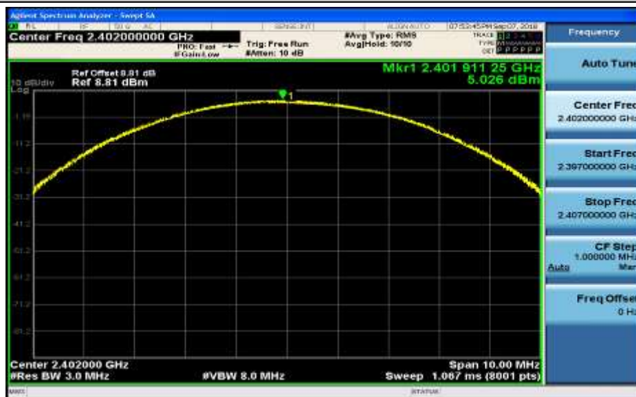
Conducted Peak Output Power_2DH5_2441
