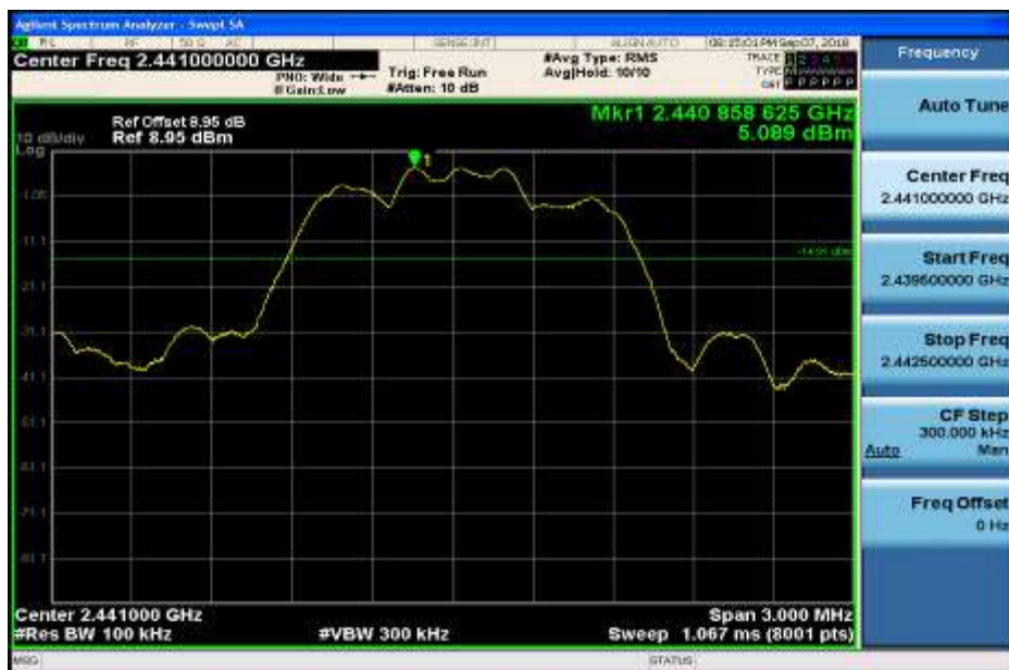
RF Conducted Spurious Emissions_3DH5_2441
