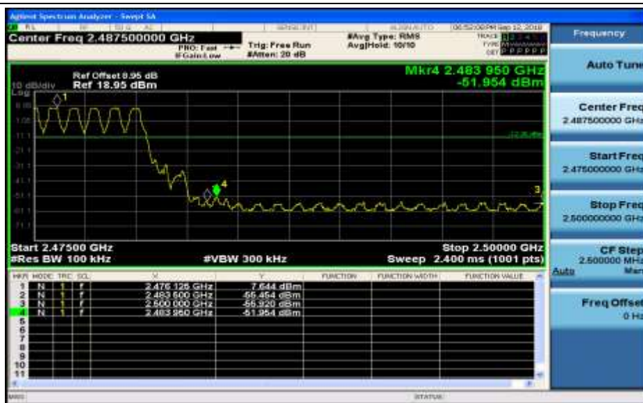
Band-edge for RF Conducted Emissions_DH5_2480_Hopping Off
