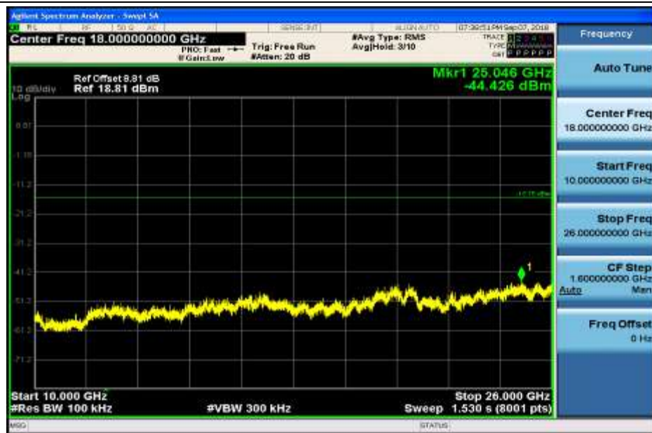
RF Conducted Spurious Emissions_DH5_2441
