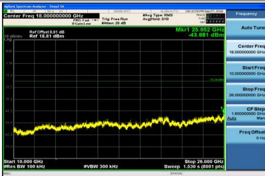
RF Conducted Spurious Emissions_3DH5_2441
