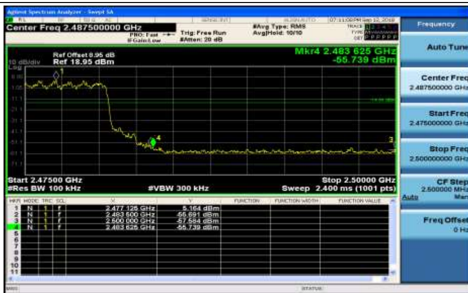
Band-edge for RF Conducted Emissions_3DH5_2480_Hopping Off
