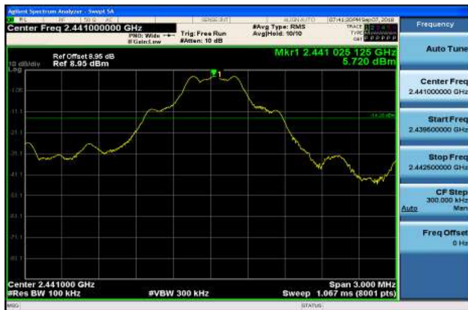
RF Conducted Spurious Emissions_DH5_2441
