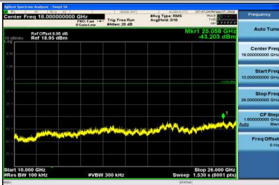
RF Conducted Spurious Emissions_2DH5_2402
