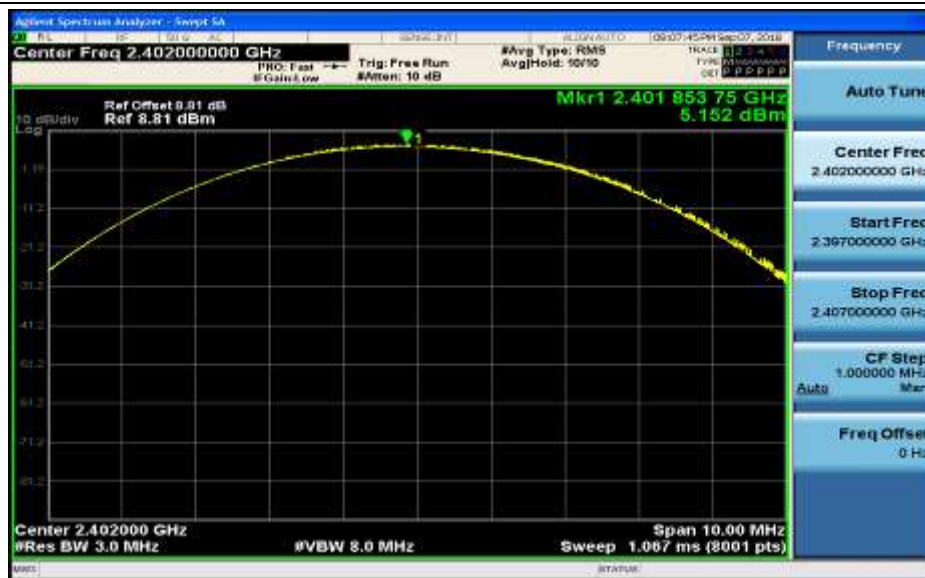
Conducted Peak Output Power_3DH5_2441
