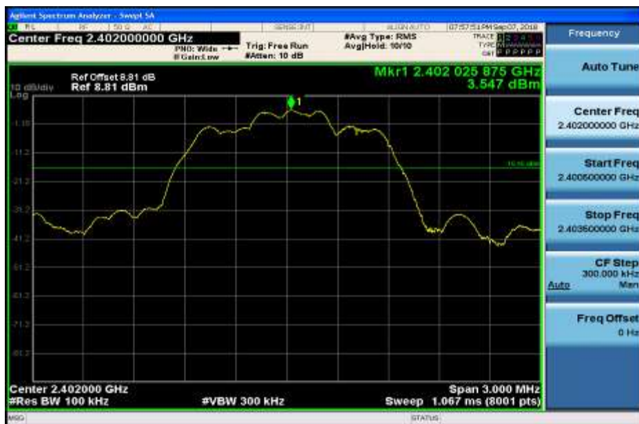
RF Conducted Spurious Emissions_2DH5_2402
