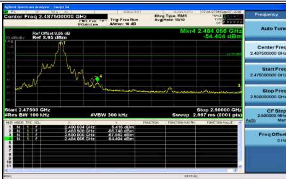
Band-edge for RF Conducted Emissions_2DH5_2402_Hopping On
