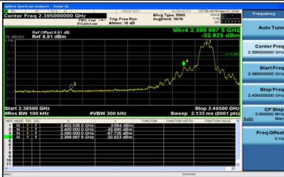
Band-edge for RF Conducted Emissions_2DH5_2480_Hopping On
