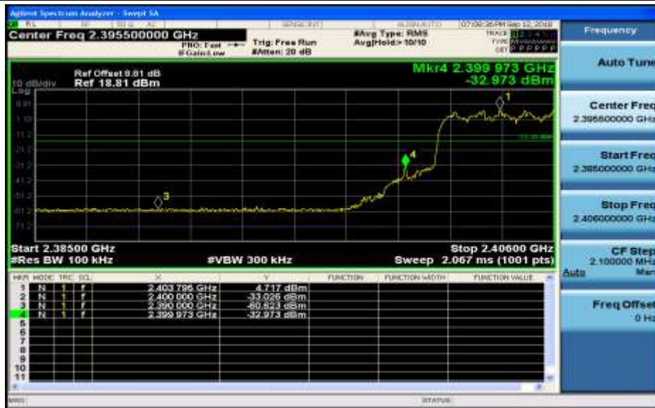
Band-edge for RF Conducted Emissions_3DH5_2402_Hopping Off
