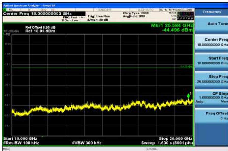
RF Conducted Spurious Emissions_DH5_2480
