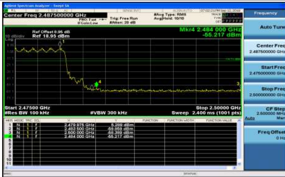
Band-edge for RF Conducted Emissions_2DH5_2480_Hopping Off
