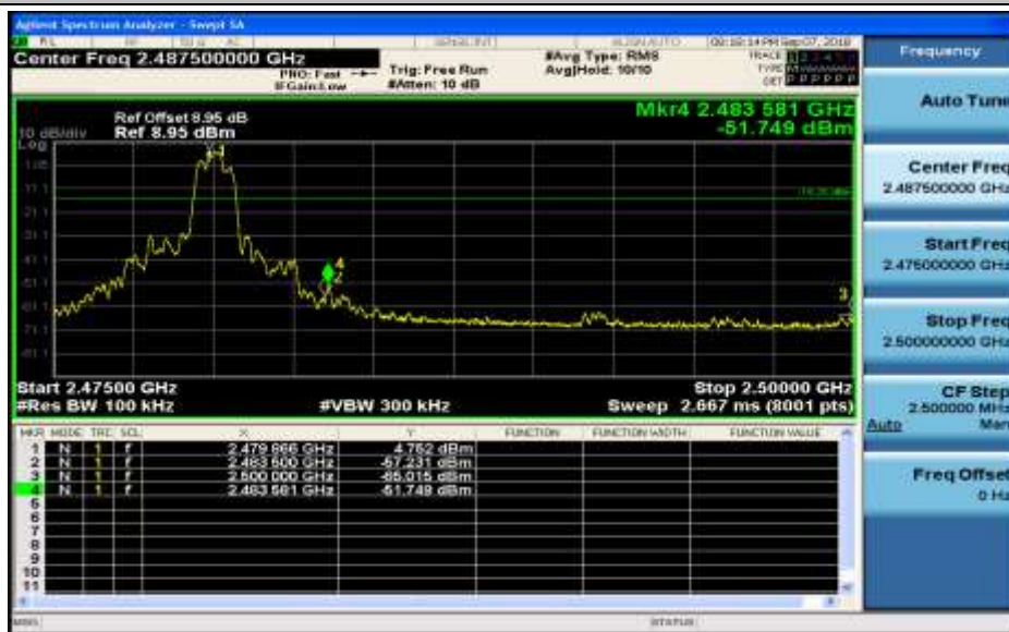
Band-edge for RF Conducted Emissions_3DH5_2480_Hopping Off
