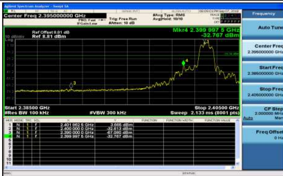
Band-edge for RF Conducted Emissions_3DH5_2480_Hopping On
