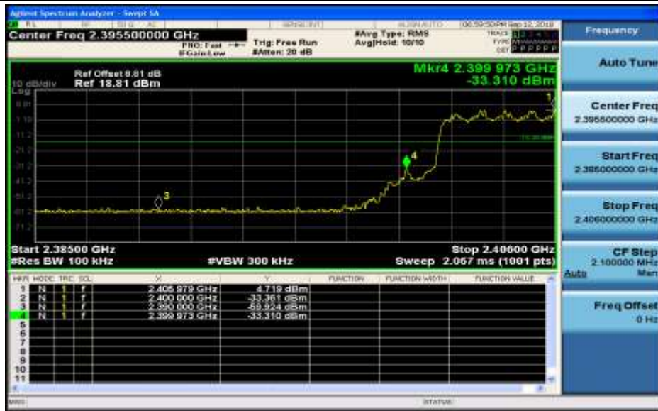
Band-edge for RF Conducted Emissions_2DH5_2402_Hopping Off
