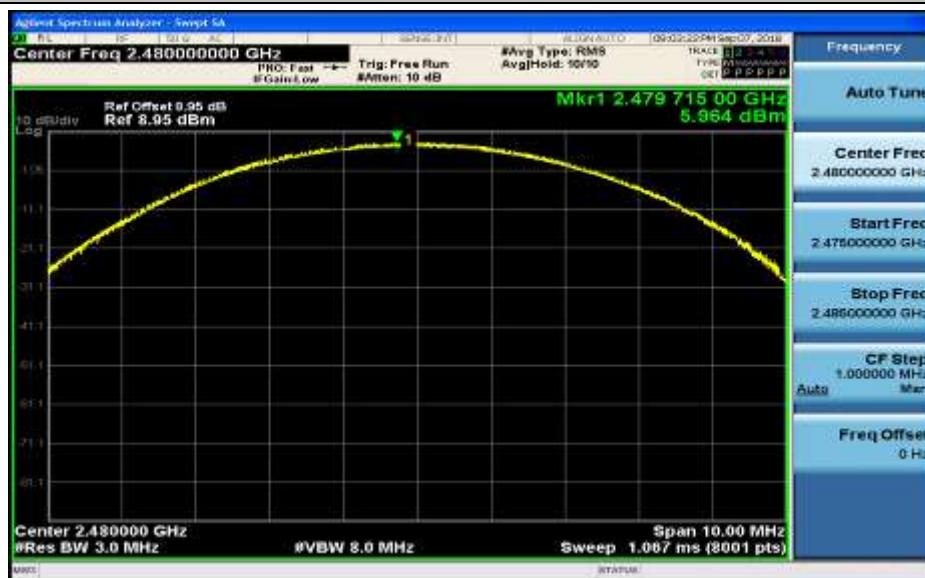
Conducted Peak Output Power_3DH5_2402
