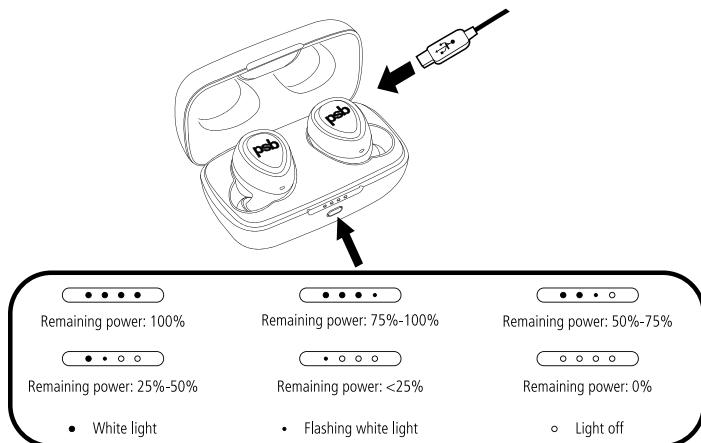
Plug in one end of the supplied USB-C charging cable to the Charging case and the other end of the USB-C charging cable to a universal 5V 1A USB-C wall adapter (not supplied).
