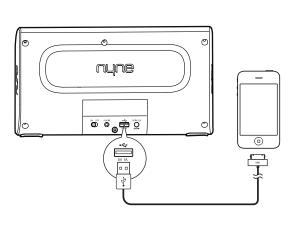
EN Charge your mobile device through the 5V USB charging socket.
