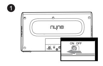
Slide the power switch to the **ON** position.
