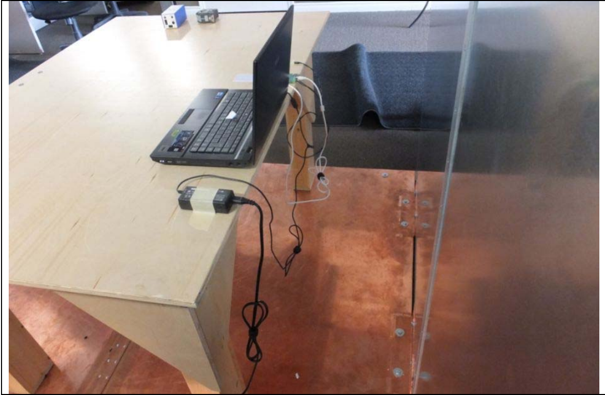
AC Power Line Conducted Emissions Setup 150 kHz – 30 MHz
