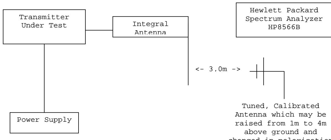
Equipment placed 80cm above ground on a rotatable platform.
