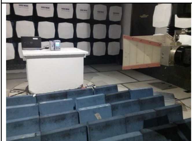
Test setup at 3 meter distance (>1GHz) - Front
