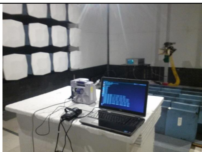
Test setup at 3 meter distance (>1GHz) - Rear
