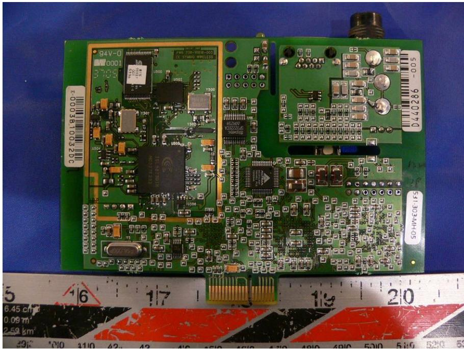
**EUT -RF Board with Shield Off Top View**
