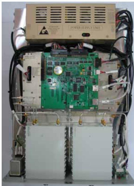
< The Inside of the Repeater >
