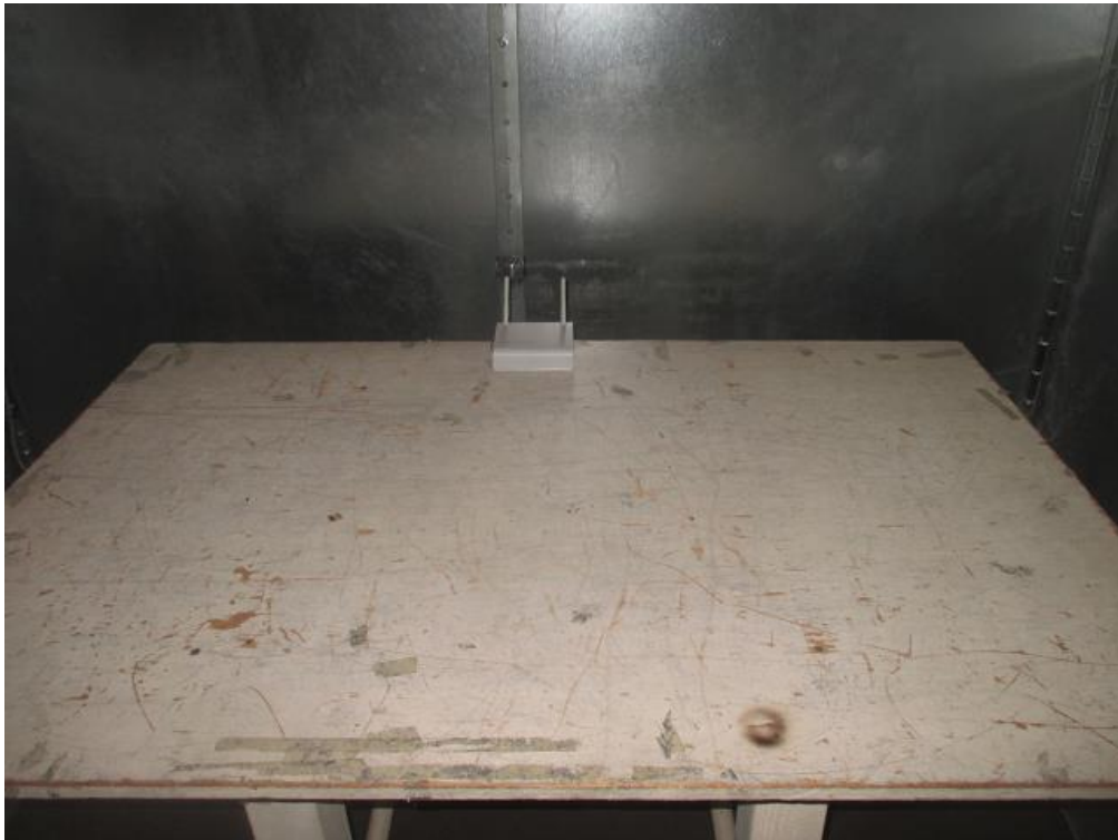
Figure 1 EUT Configuration for Radiated & Conducted Emission Tests
