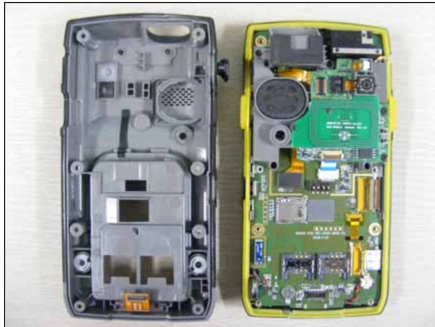
Top view of Main PCB
