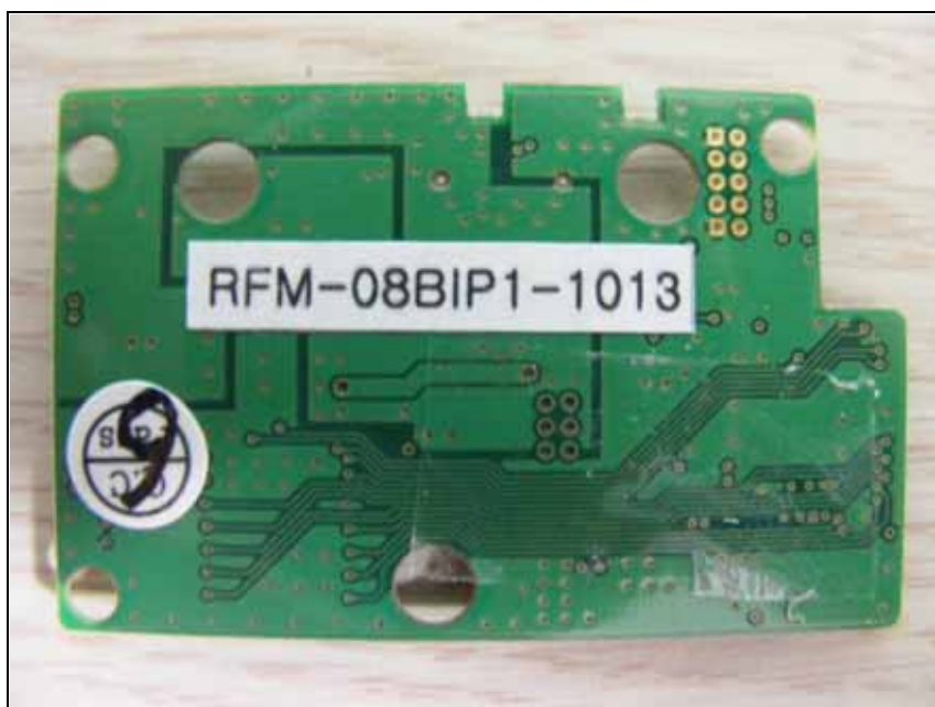
Bottom of Sub- PCB
