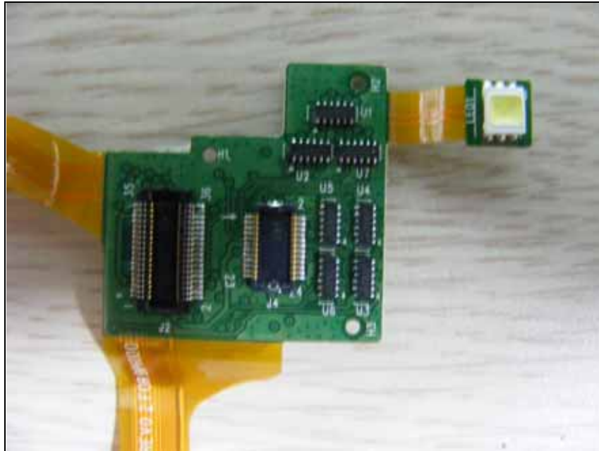
Bottom of Sub- PCB
