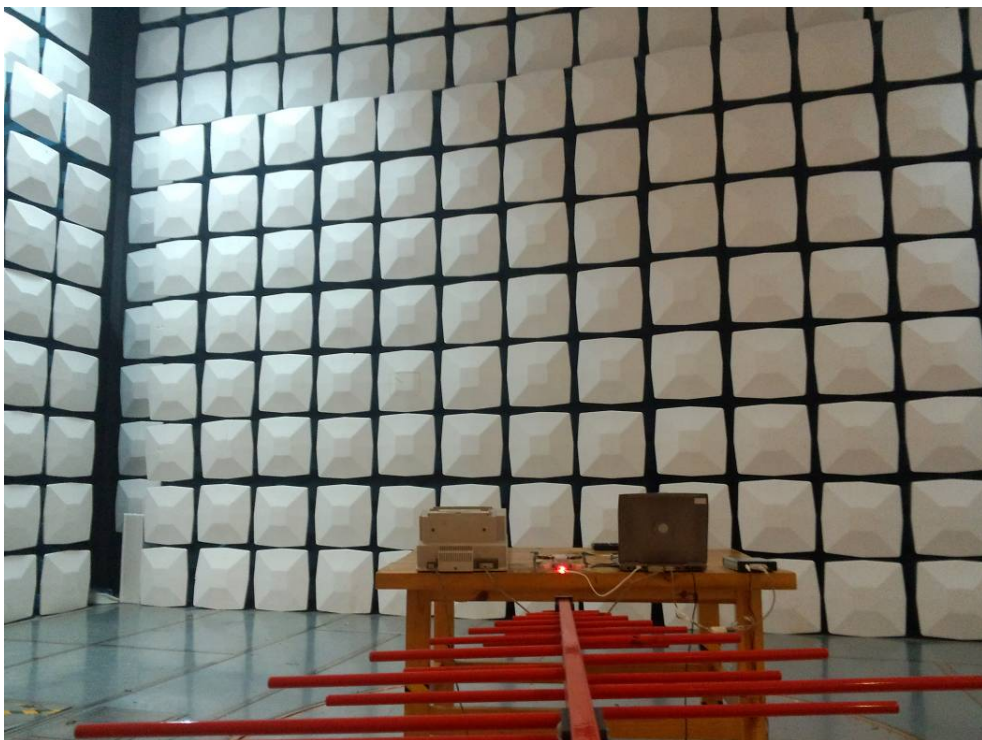
Radiated Emission Below 1GHz – Rear View
