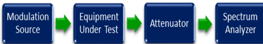
Figure 2: Modulation Characteristics Bandwidth Test Setup
