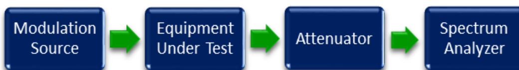
Figure 3: Occupied Bandwidth Test Setup
