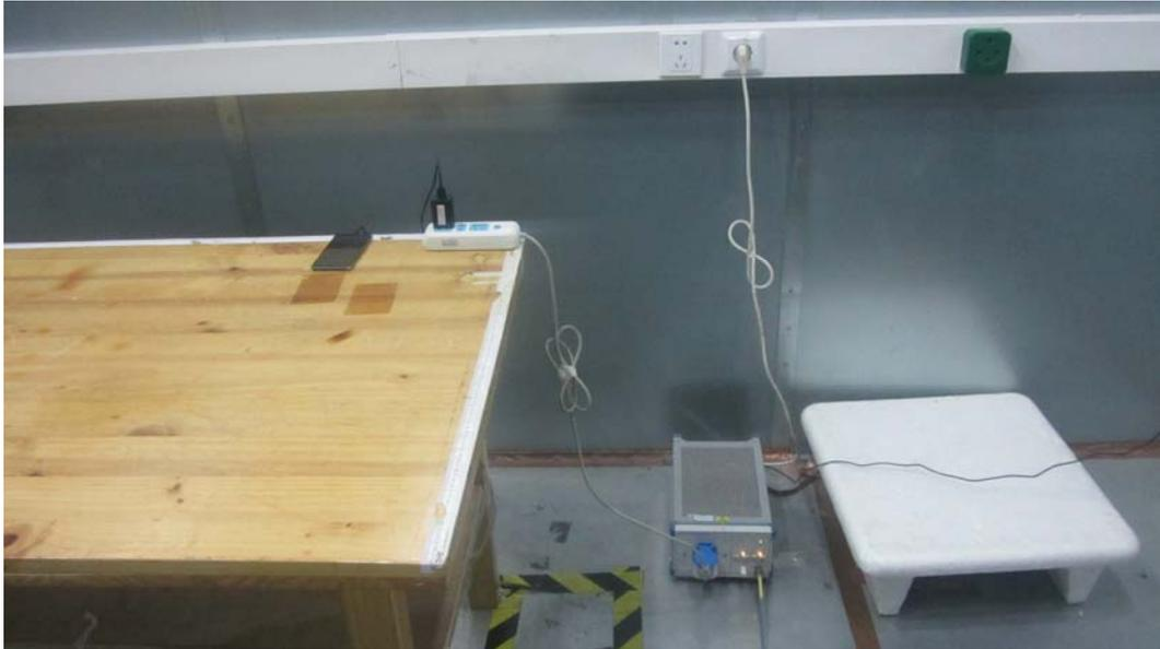
**Picture 3 Conducted Emission Test Setup**
