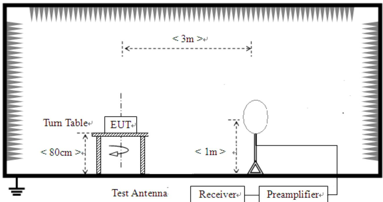
For radiated emissions from 30MHz to 1GHz
