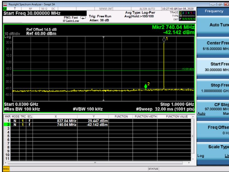
EDGE 850MHz Channel = 190, 30MHz to 1GHz
