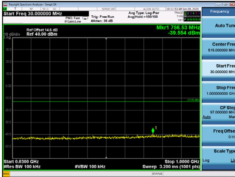
EDGE 1900MHz Channel = 512, 30MHz to 1GHz
