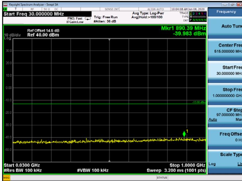
GSM 1900MHz Channel = 661, 30MHz to 1GHz
