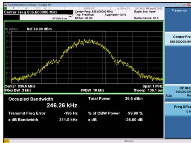
(Plot A2: GSM 850MHz Channel = 190 Occupied bandwidth)
