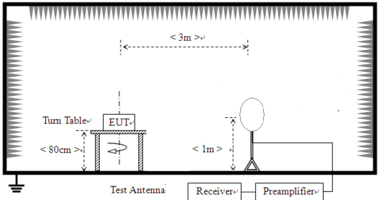
For radiated emissions from 30MHz to 1GHz
