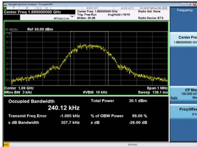
(Plot D2: EDGE 1900MHz Channel = 661 Occupied bandwidth)
