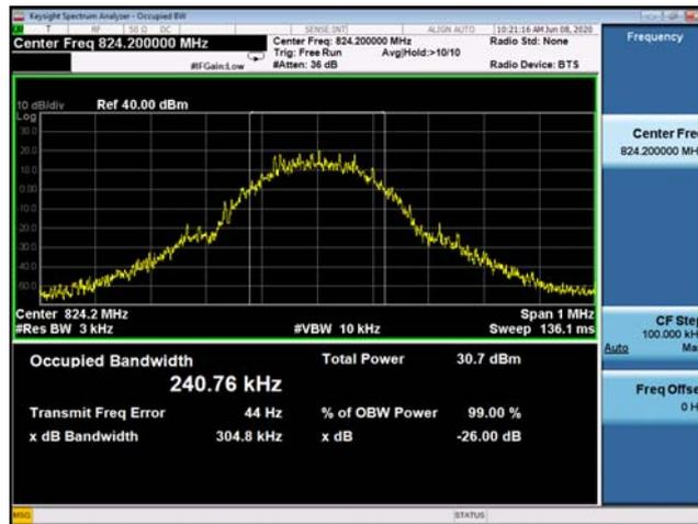
(Plot C1: EDGE 850MHz Channel = 128 Occupied bandwidth)
