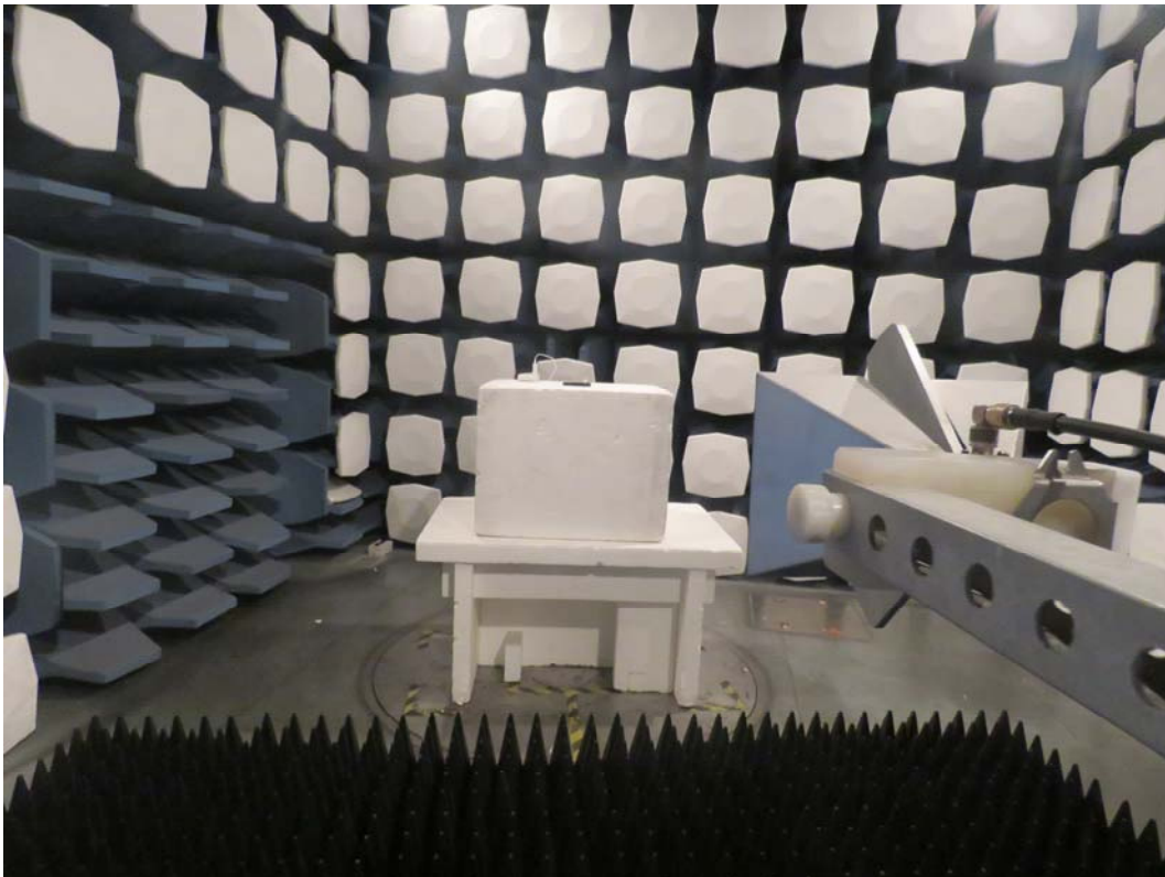
Picture 2 Radiated Emission Test Setup
