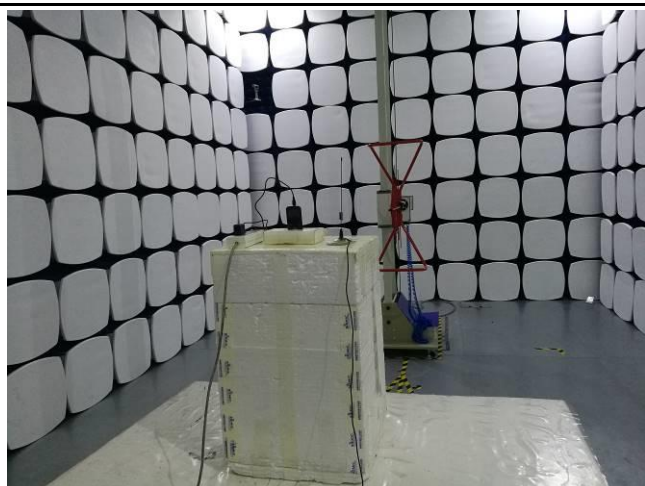
Radiated Spurious Emissions Test Setup Below 1GHz
