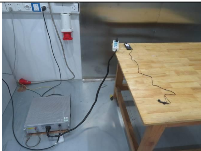
Conducted Emissions Test Setup Front View
