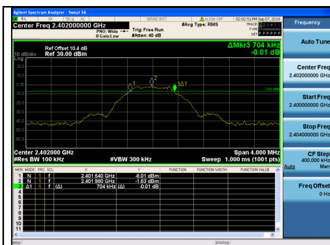
6dB Bandwidth - Low CH 2402
