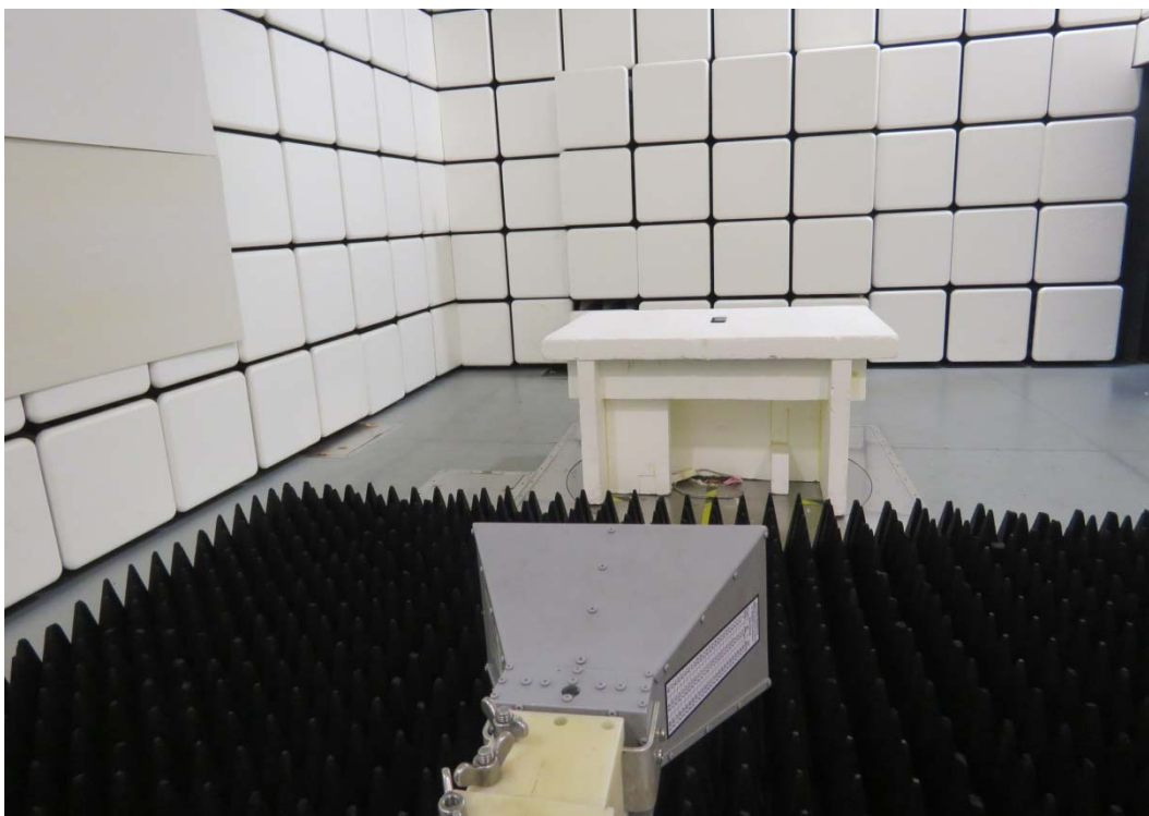
Picture 1: Radiated Spurious Emissions Test setup
