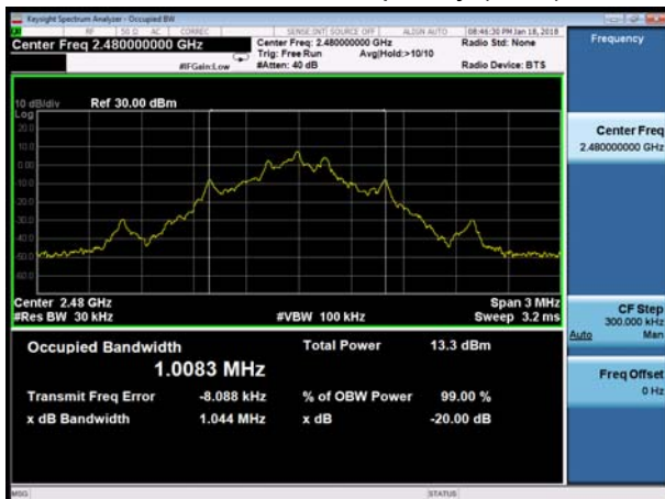
BT DH5 CH78, Carrier frequency (MHz): 2480
