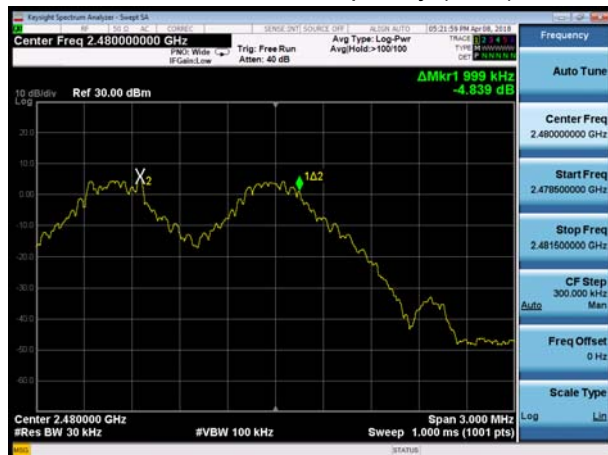
BT DH5 CH78, Carrier frequency (MHz): 2480
