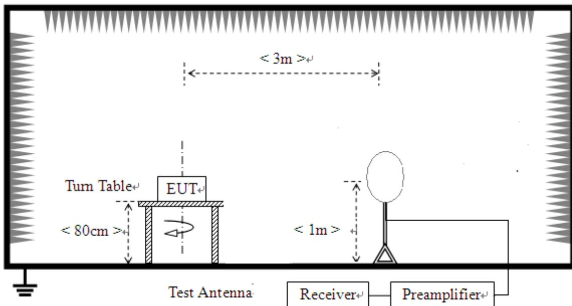
**For radiated emissions from 30MHz to 1GHz**
