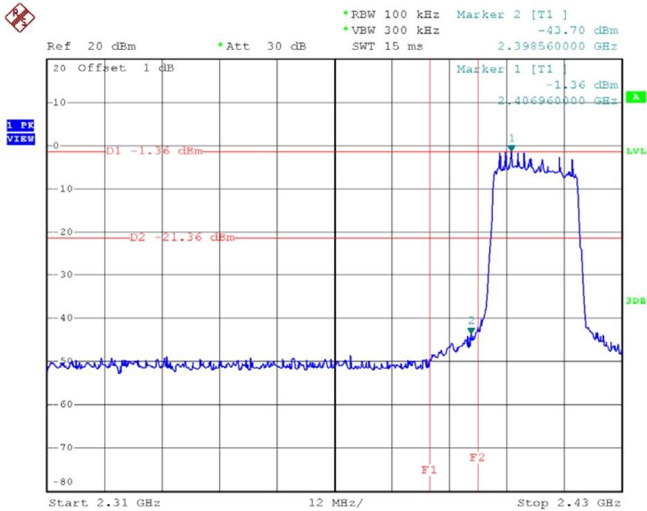
802.11n20 - Low Band Edge Plot on Channel 1
