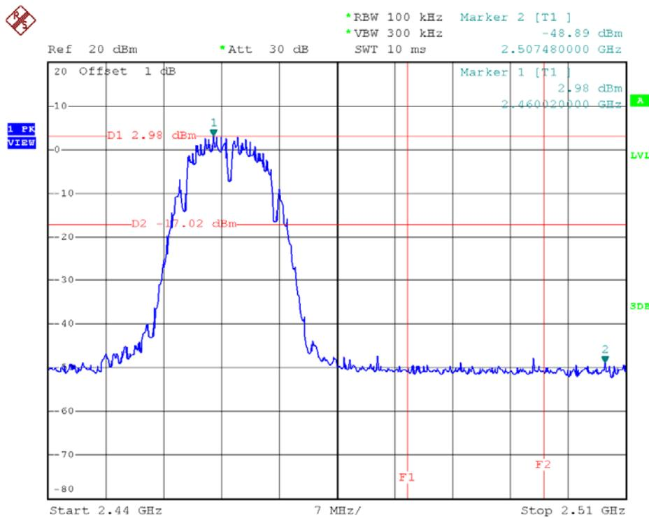
802.11b - High Band Edge Plot on Channel 11
