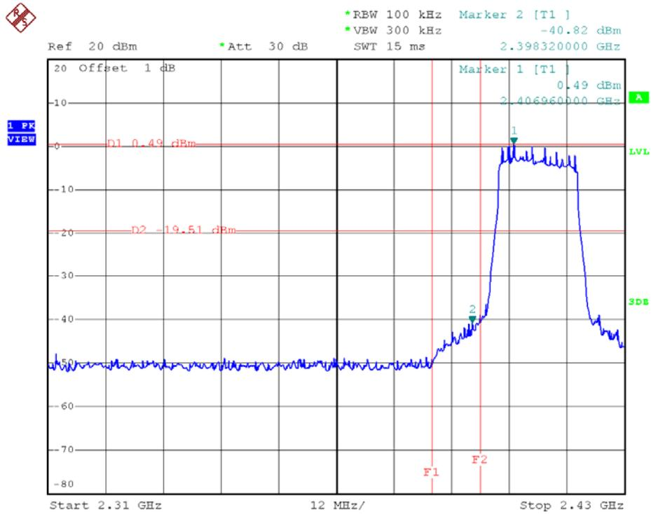
802.11g - Low Band Edge Plot on Channel 1
