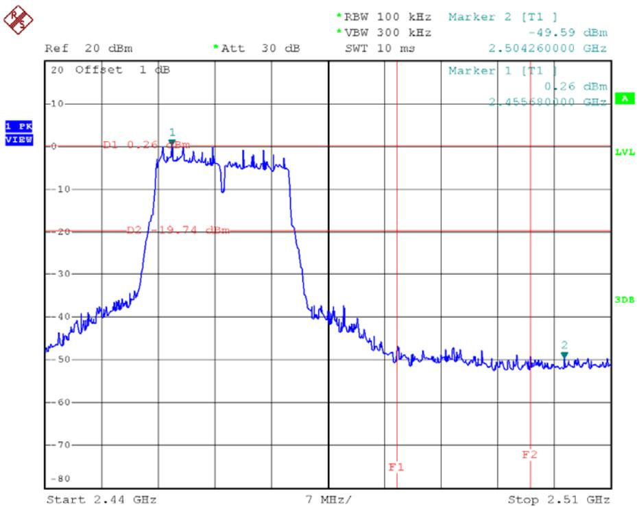
802.11g - High Band Edge Plot on Channel 11
