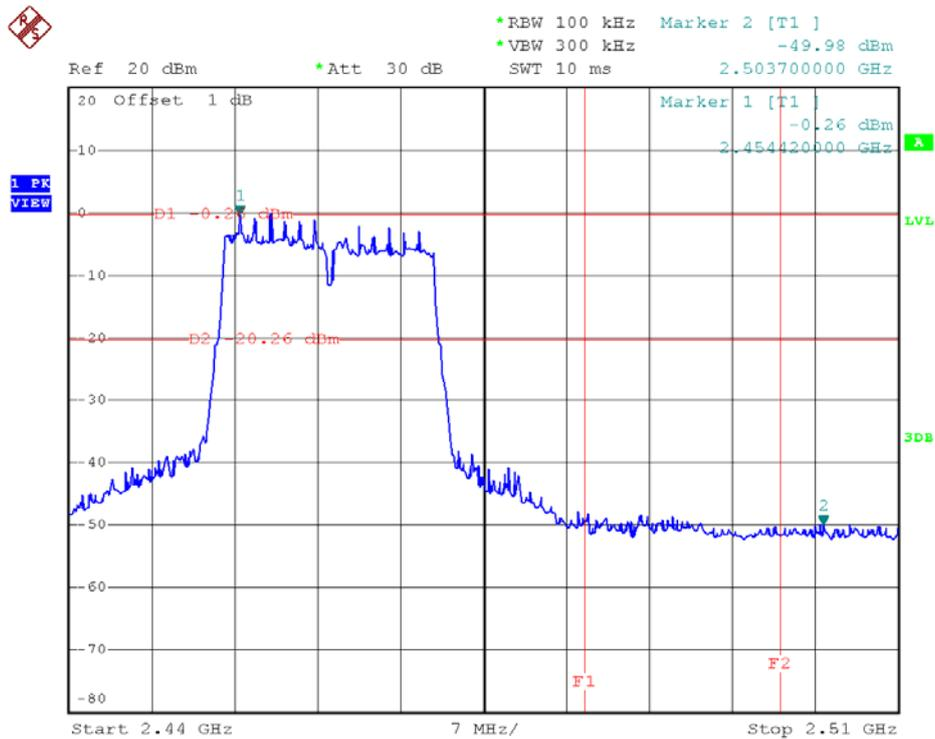
802.11n20 - High Band Edge Plot on Channel 11
