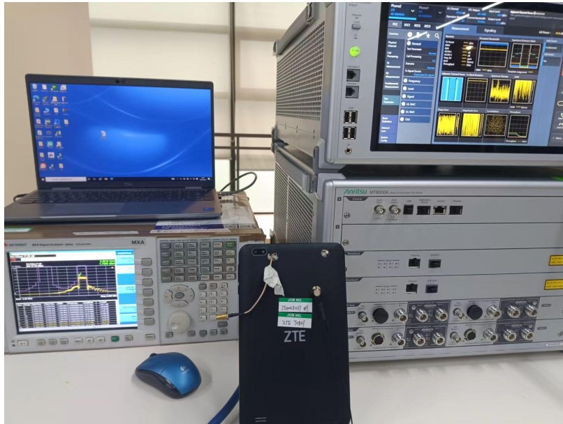
'RF Conducted Test setup (GSM/WCDMA/LTE)
