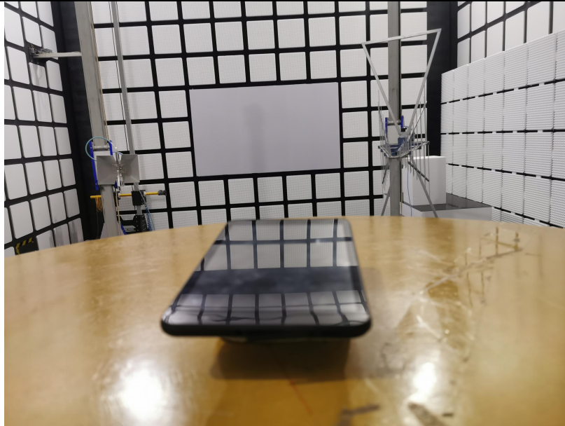
Spurious Radiated Emissions Test setup
