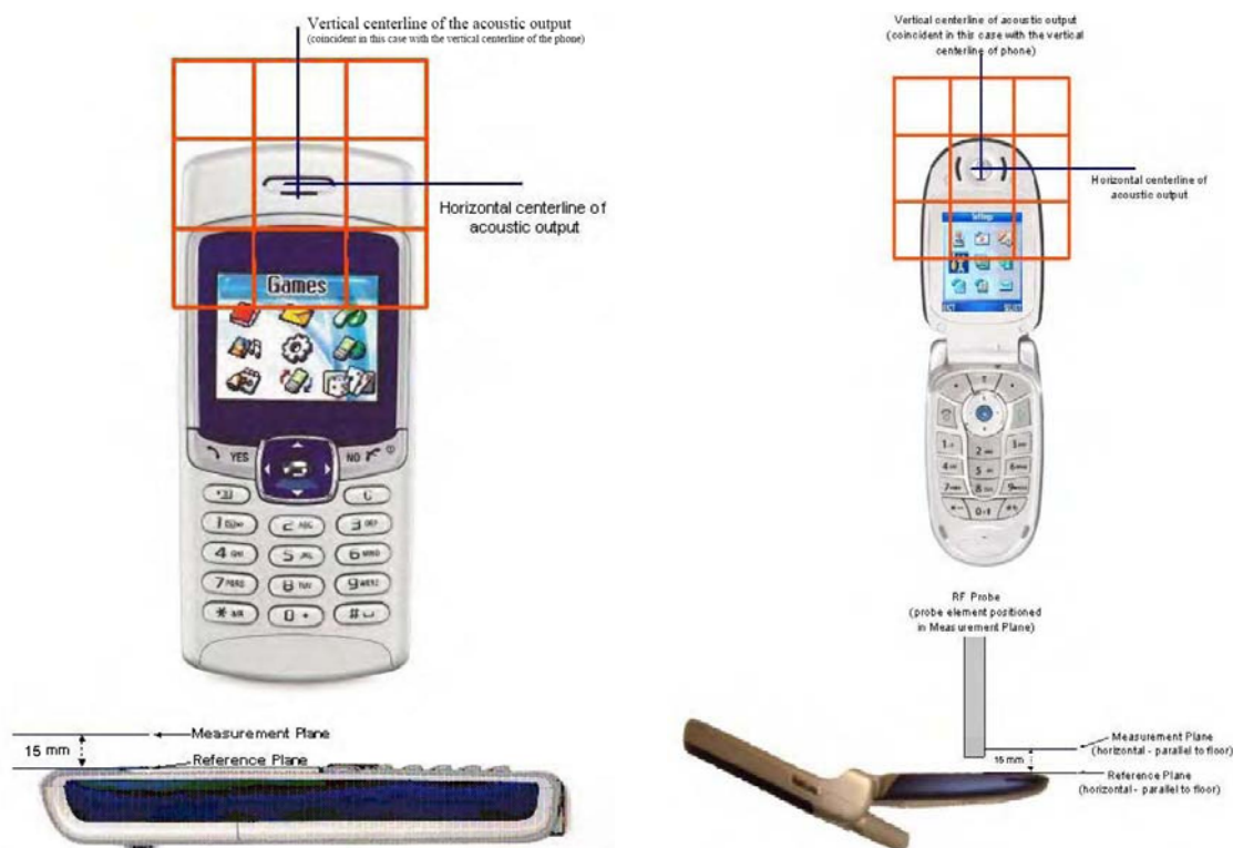
Fig 9.1 A typical EUT reference and plane for HAC measurements
