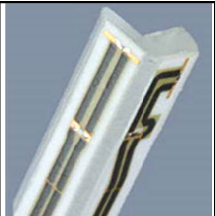
Fig 5.2 Photo of E-field Probe
