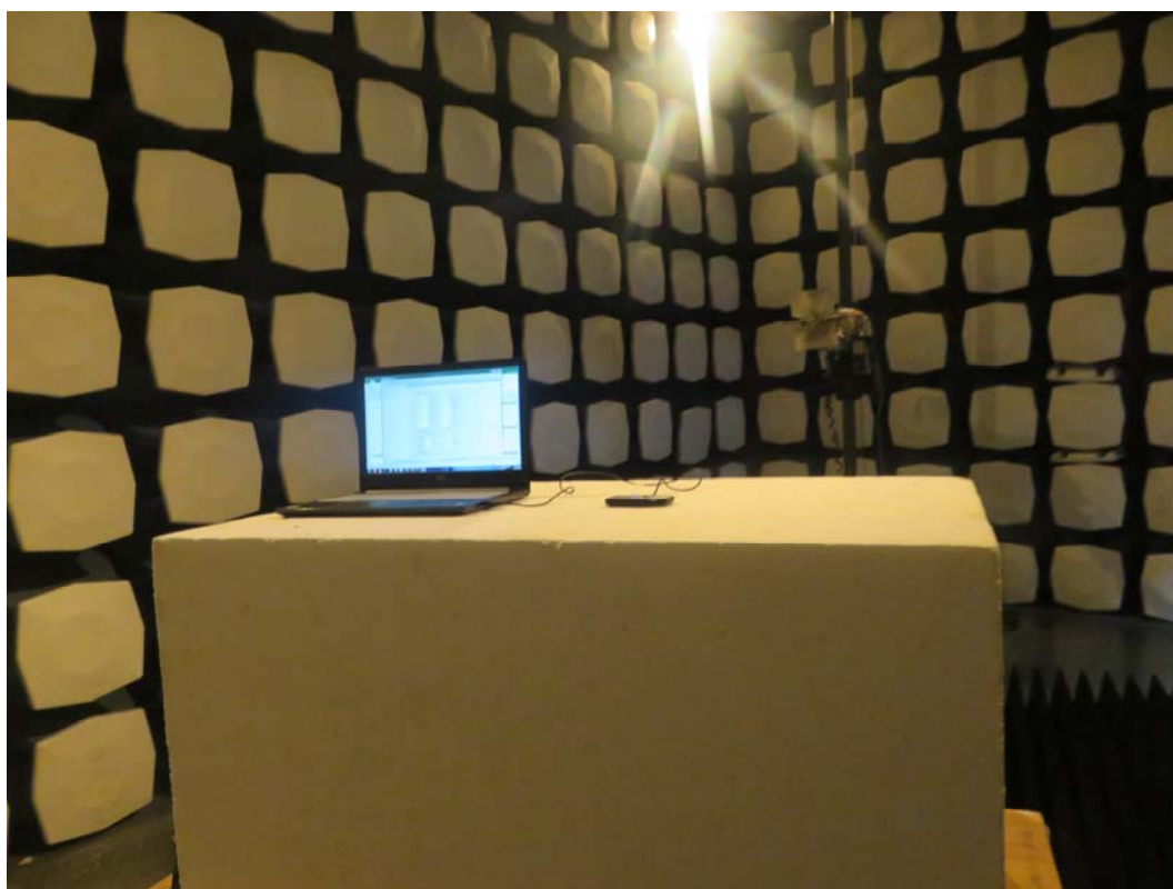
Picture 1: Radiated Spurious Emissions Test setup
