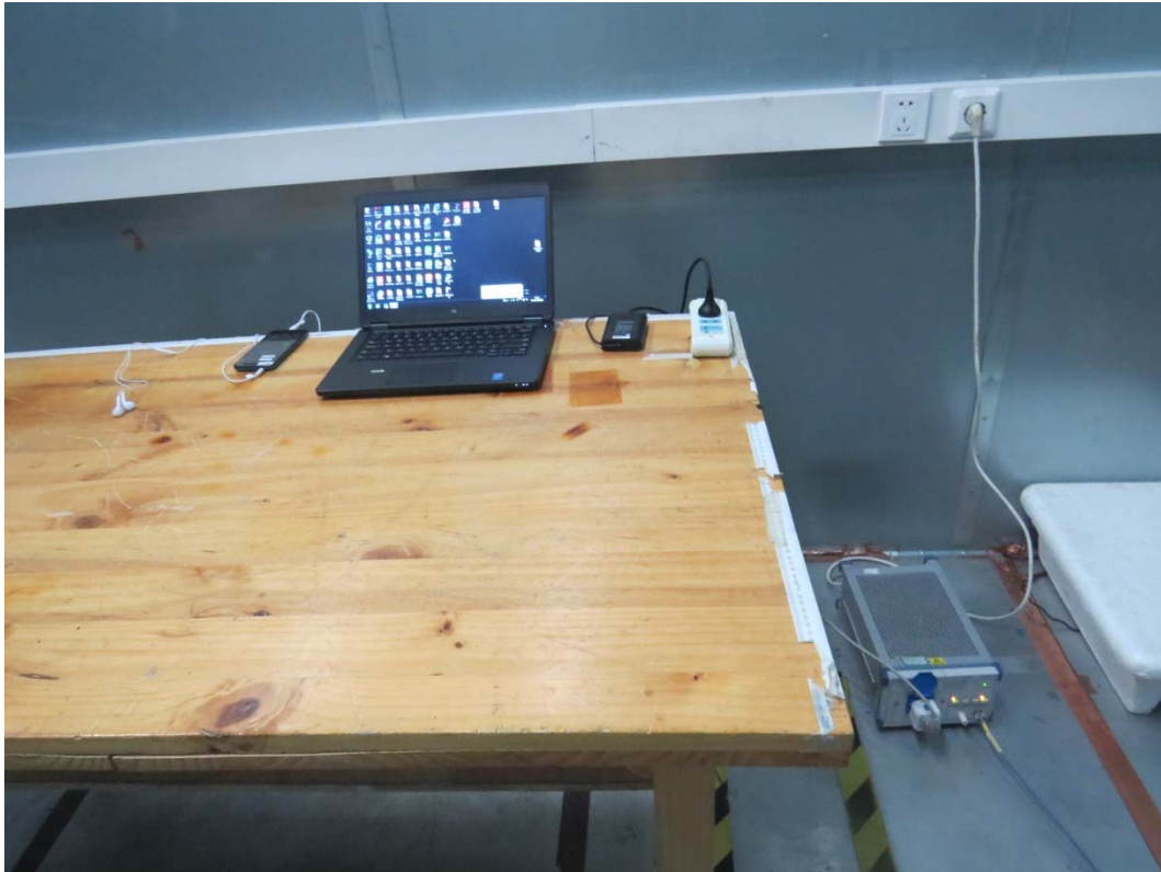
Picture 2 Conducted Emission Test Setup
