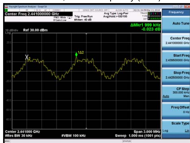
BT 3DH5 CH39, Carrier frequency (MHz): 2441
