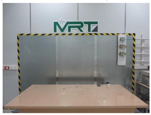
Description: Back View of the Conducted Emission Test Setup for  $0.15 kHz \sim 30 MHz$
