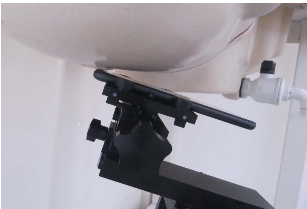
Picture 4: Right Hand Tilt 15 Degree Position
