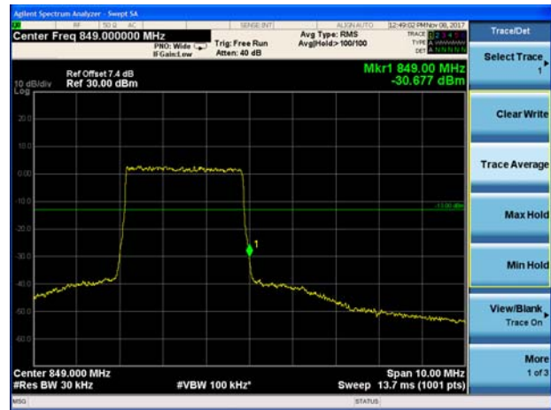
LTE Band 5 16QAM 5MHz CH-High 1RB
