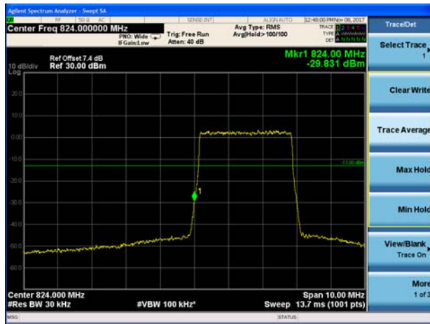
LTE Band 5 16QAM 5MHz CH-Low 1RB
