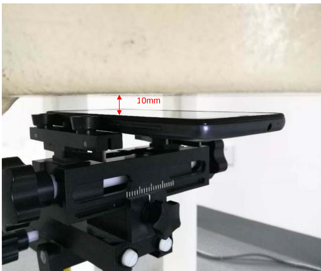
Picture 6: Front Side, the distance from handset to the bottom of the Phantom is 10mm
