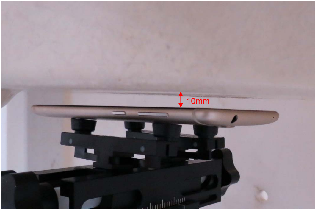
Picture 20: Front Side, the distance from handset to the bottom of the Phantom is 10mm
