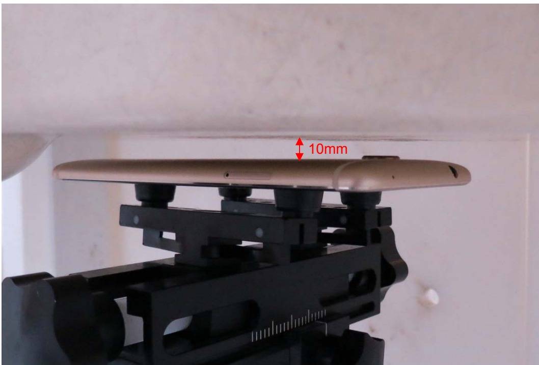
Picture 19: Back Side, the distance from handset to the bottom of the Phantom is 10mm
