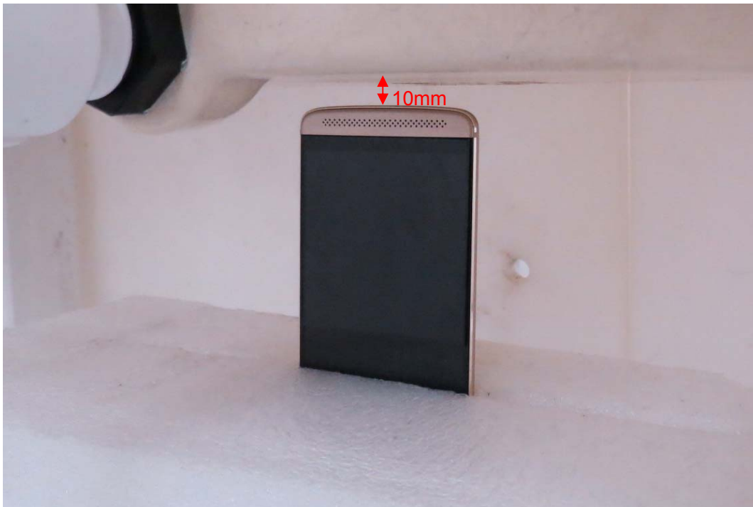
Picture 21: Bottom Side, the distance from handset to the bottom of the Phantom is 10mm
