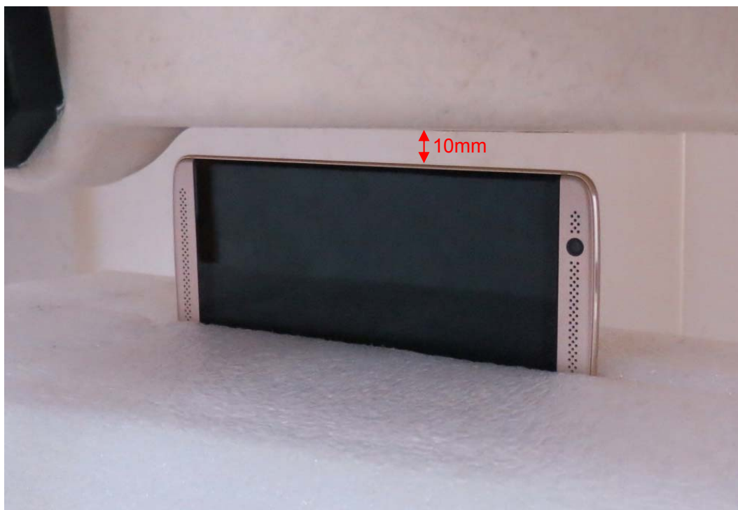
Picture 22: Left Side, the distance from handset to the bottom of the Phantom is 10mm
