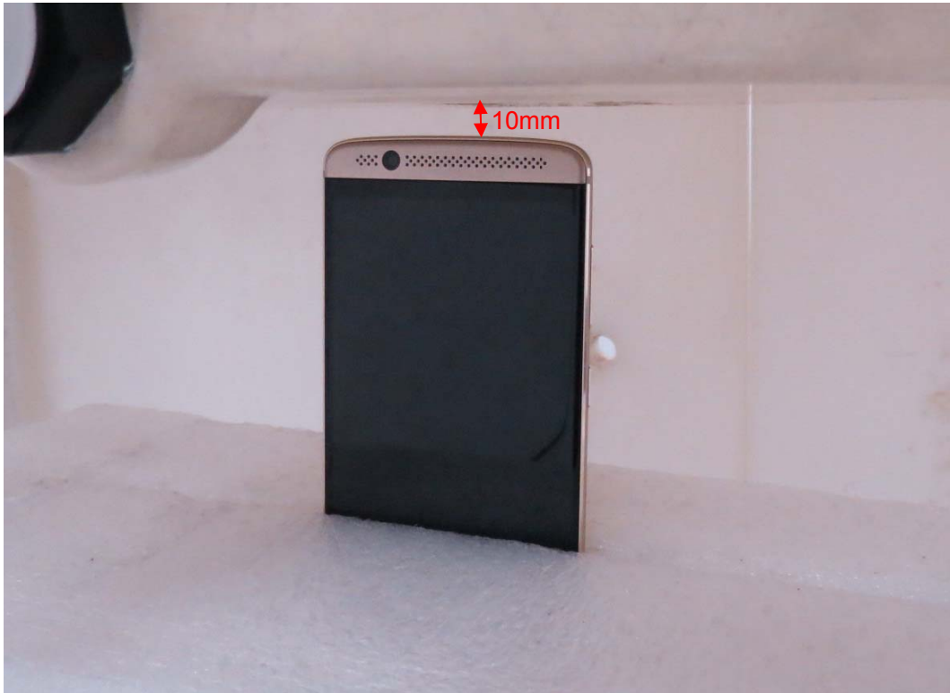
Picture 24: Top Side, the distance from handset to the bottom of the Phantom is 10mm
