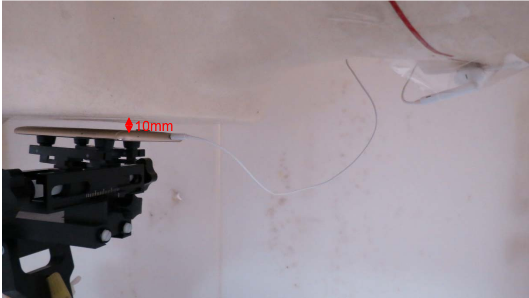
Picture 26: Back Side with Earphone, the distance from handset to the bottom of the Phantom is 10mm
