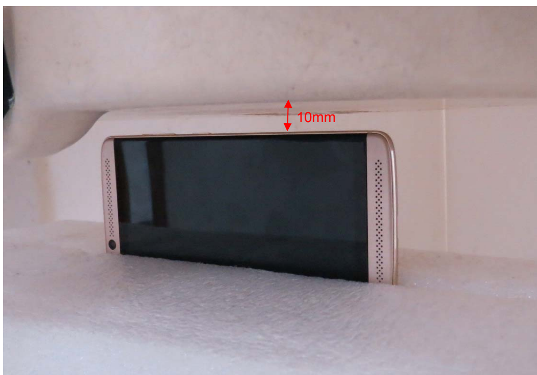
Picture 23: Right Side, the distance from handset to the bottom of the Phantom is 10mm
