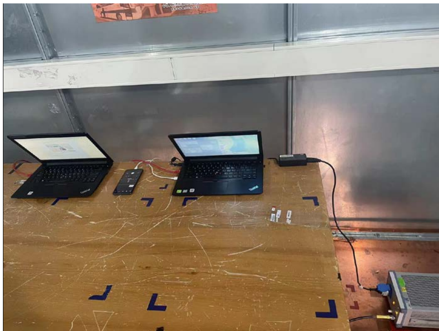
Conducted Emissions Test Setup
