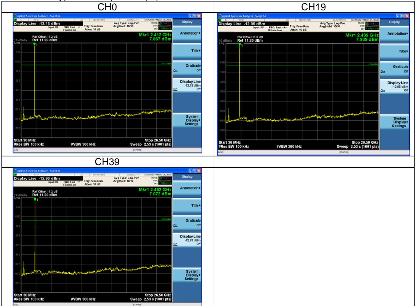
**Band edge measurement (RF Conducted measurement)**
