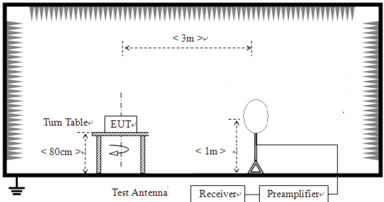
For radiated emissions from 30MHz to 1GHz
