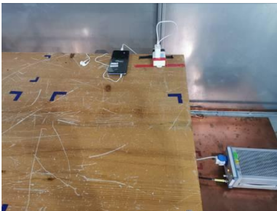
Conducted Emissions Test Setup (with charger)
