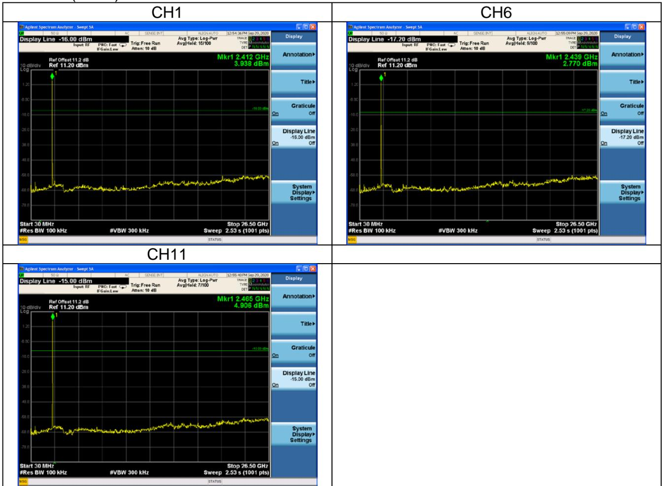
**Band edge measurement (RF Conducted measurement)**
