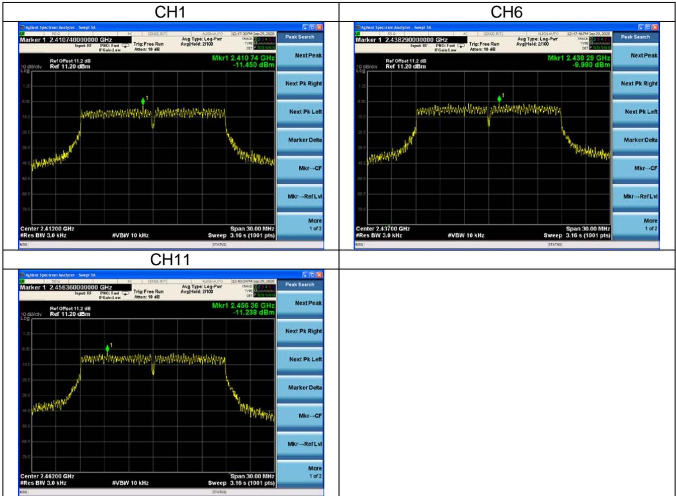
**Conducted Out of band emission measurement**
