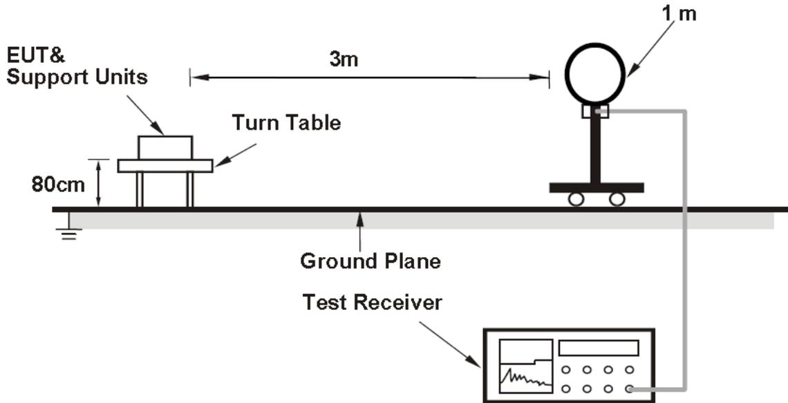
For Radiated emission 30MHz to 1GHz
