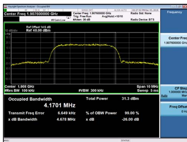
(Plot F3: WCDMA 1900MHz Channel = 9538 Occupied bandwidth)
