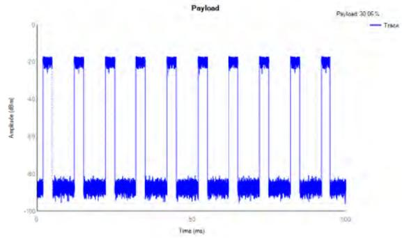
LTE Band 40 Subset 2 64QAM 5MHz CH-Middle
