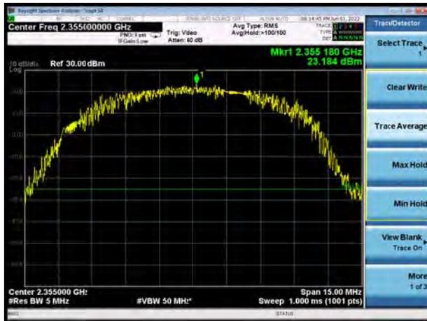
LTE Band 40 Subset 2 64QAM 5MHz CH-High
