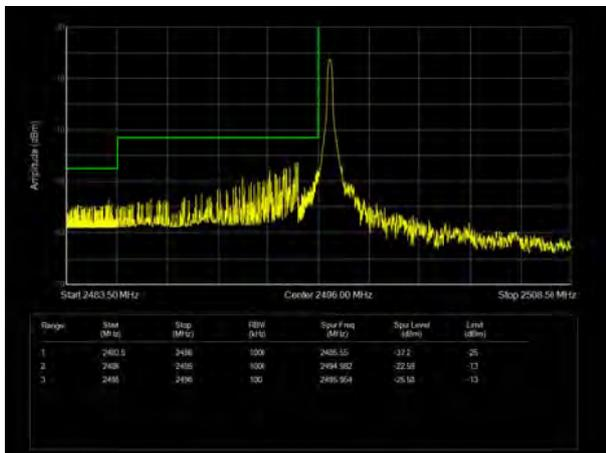
LTE Band 41 16QAM 10MHz CH-High, 1 RB
