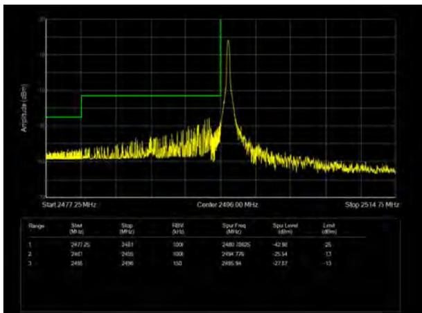
LTE Band 41 64QAM 15MHz CH-High, 1 RB
