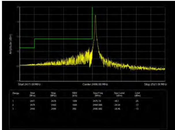
LTE Band 41 64QAM 20MHz CH-High, 1 RB
