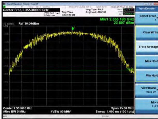
LTE Band 40 Subset 2 16QAM 5MHz CH-High
