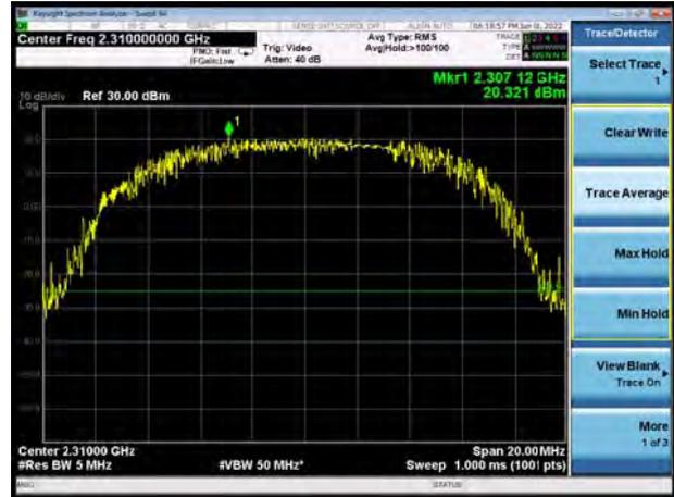
LTE Band 40 Subset 1 QPSK 5MHz CH-Middle
