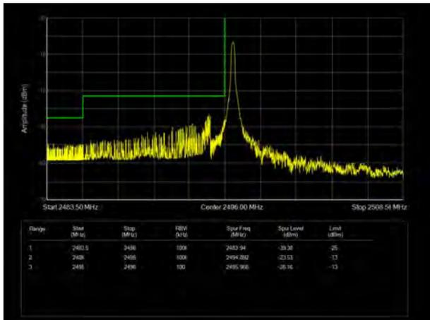
LTE Band 41 64QAM 10MHz CH-High, 1 RB
