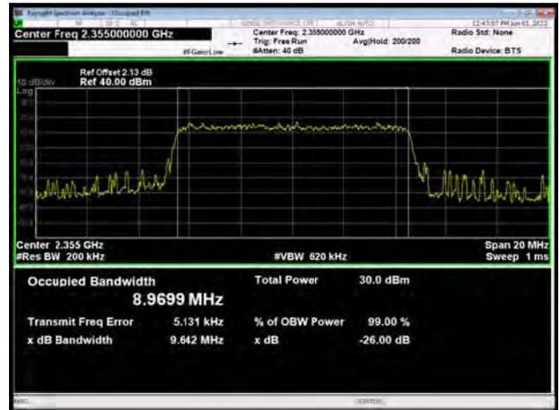
LTE Band 40 Subset 2 QPSK 5MHz CH-Middle
