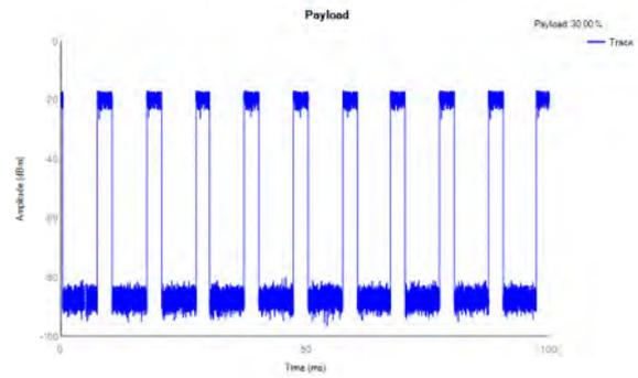
LTE Band 40 Subset 1 QPSK 5MHz CH-Middle
