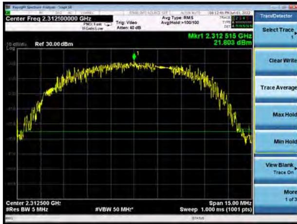
**Power Spectral Density (dBm/MHz)**
