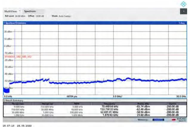
NR n2 P1/2 BPSK 20MHz CH-High 9kHz~20GHz
