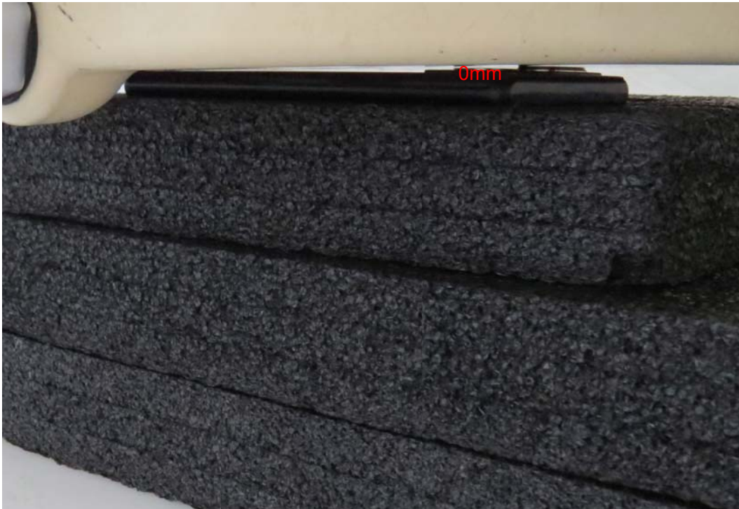
Picture 13: Back Side, the distance from handset to the bottom of the Phantom is 0mm
