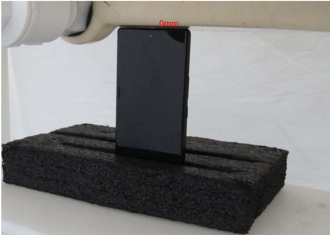
Picture 17: Top Edge, the distance from handset to the bottom of the Phantom is 0mm
