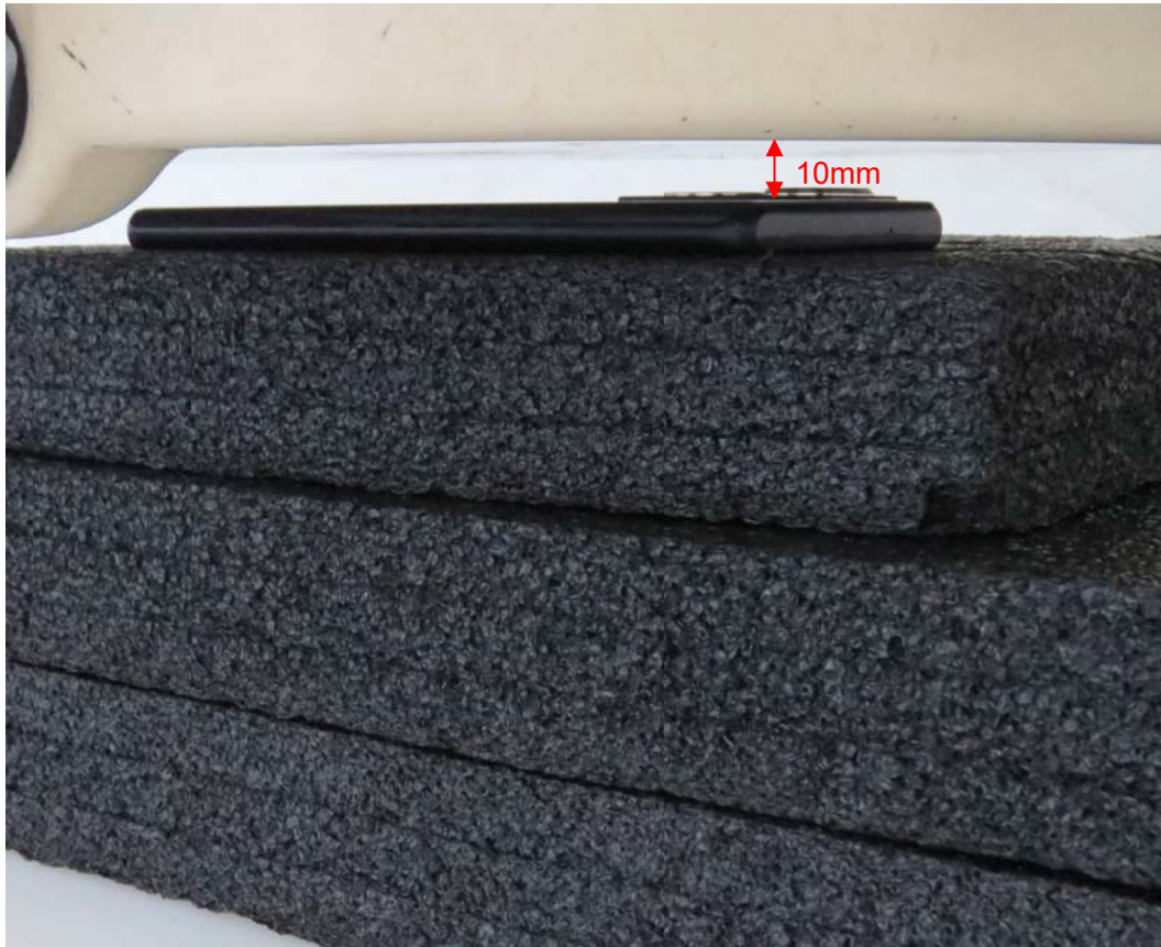
Picture 7: Back Side, the distance from handset to the bottom of the Phantom is 10mm
