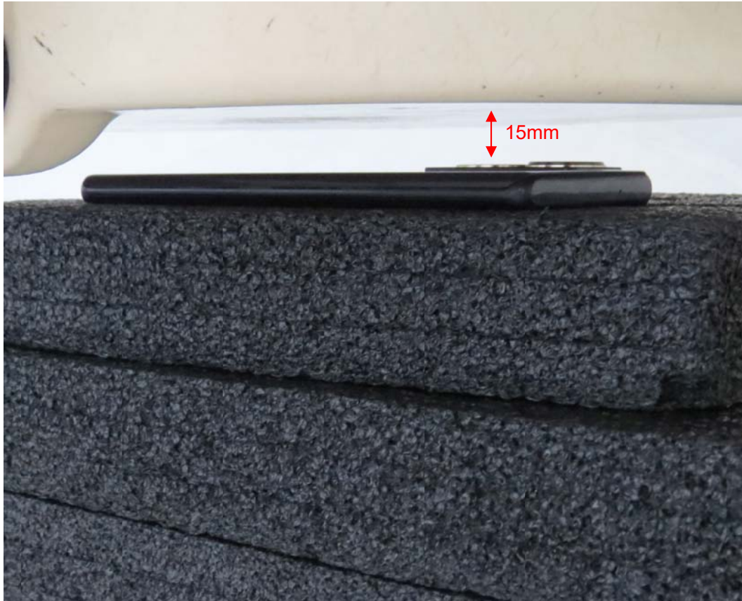
Picture 5: Back Side, the distance from handset to the bottom of the Phantom is 15mm
