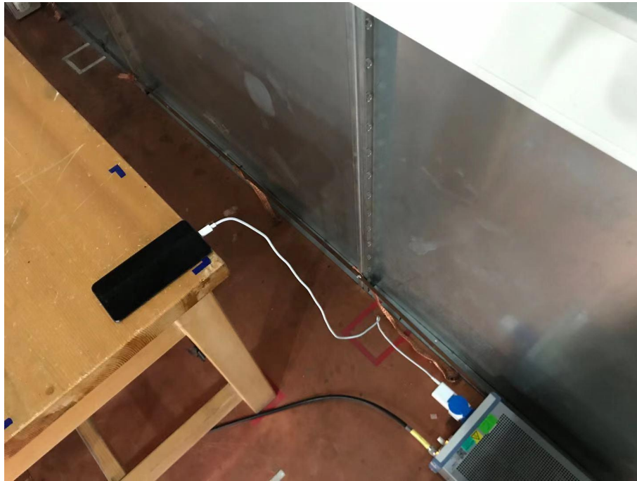
Conducted Emissions Test Setup (with charger)
