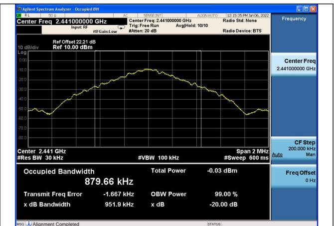
Test Mode:GFSK(DH5) MHz
