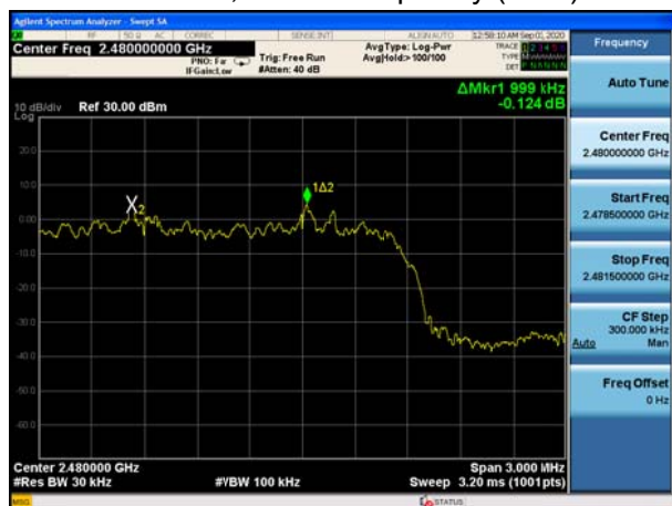
BT 2DH5 CH78, Carrier frequency (MHz): 2480
