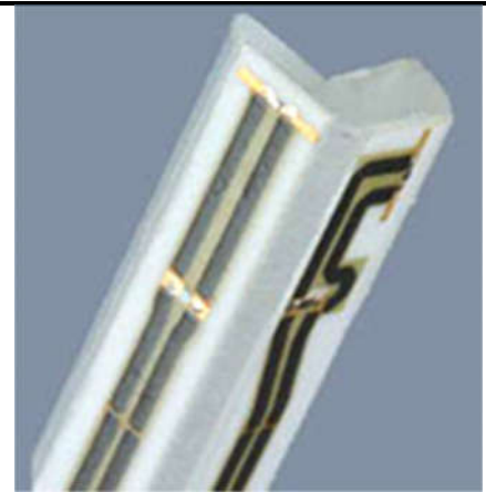
Fig 5.2 Photo of E-field Probe
