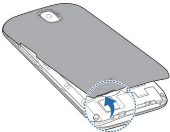
2. Hold the microSDHC card with the cut corner oriented as shown and slip it into the card slot.
